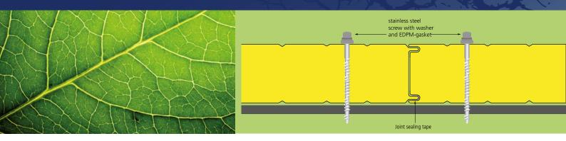
The Metfiber® Eco Wall panel with glass wool core fulfils all the requirements for non-combustible building materials. The glass wool used in this product consists of 80% recycled material, contributing significantly to the saving of natural resources and making the product an ecological building material. The deadweight of the panel is distinctly lower than that of conventional sandwich panels with rock wool insulation core, hence enabling an easier, faster
