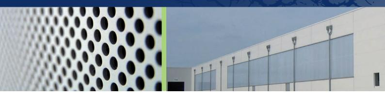
Hipertec® Wall Sound is a sandwich panel with an insulation core of mineral wool and steel cover sheets, the internal sheet being perforated. This panel is perfectly apt for buildings with high requirements for noise insulation and sound absorption. The design of the internal sheet improves room acoustics substantially. This system patented by Metecno applies a special fleece as trickle protection between the internal sheet and the rock wool core.
