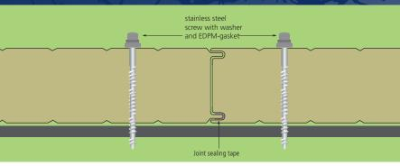
Hipertec® Wall is a sandwich panel with non-combustible insulation core of rock wool and suits best to meet today's high requirements for fire protection and sound insulation. Depending on the core thickness the fire resistance may reach up to 120 minutes. High support widths and an easy installation -both vertical and horizontal- make this product very cost effective, perfectly apt for application as separation
