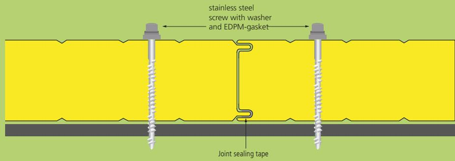
The Metfiber® Eco Wall panel with glass wool core fulfills all the requirements for non-combustible building materials. The glass wool used in this product consists of 80% recycled material, contributing significantly to the saving of natural resources and making the product an ecological building material. The deadweight of the panel is distinctly lower than that of conventional sandwich panels with rock wool insulation core, hence enabling an easier, faster
