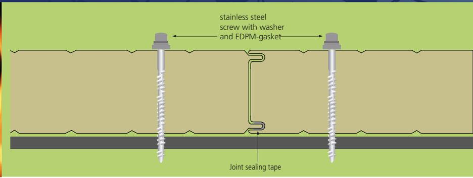
Hipertec® Wall is a sandwich panel with non-combustible insulation core of rock wool and suits best to meet today's high requirements for fire protection and sound insulation. Depending on the core thickness the fire resistance may reach up to 120 minutes. High support widths and an easy installation -both vertical and horizontal- make this product very cost effective, perfectly apt for application as separation
