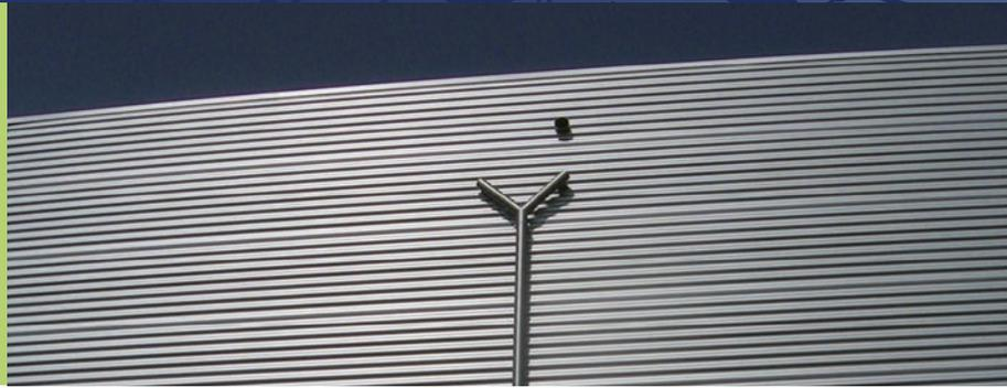
This sandwich panel with sinus corrugated external sheet and hidden fixing is a great esthetical option for modern facades by giving them a lively touch with its original wave design. The highly heat insulating CFC and HCFC free polyurethane rigid foam core suits best for today's requirements for thermal insulation and moisture protection. A non-displaceable sealing strip foamed into the longitudinal joint procures resistance to driving rain
