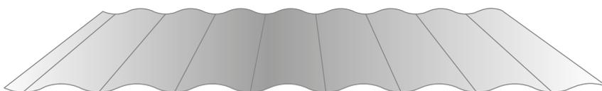
Side A: 25 µm Polyester coating with protective film / Side B: RSL-protective lacquer / lengths: 2.000 mm to 7.500 mm (other lengths on request) / sheet thicknesses: 0,50 mm, 0,60 mm, 0,75 mm
