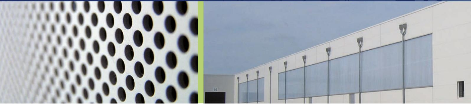
Hipertec® Wall Sound is a sandwich panel with an insulation core of mineral wool and steel cover sheets, the internal sheet being perforated. This panel is perfectly apt for buildings with high requirements for noise insulation and sound absorption. The design of the internal sheet improves room acoustics substantially. This system patented by Metecno applies a special fleece as trickle protection between the internal sheet and the rock wool core.
