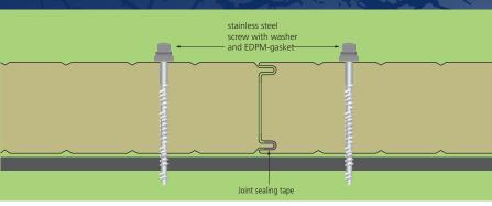
Hipertec® Wall is a sandwich panel with non-combustible insulation core of rock wool and suits best to meet today's high requirements for fire protection and sound insulation. Depending on the core thickness the fire resistance may reach up to 120 minutes. High support widths and an easy installation -both vertical and horizontal- make this product very cost effective, perfectly apt for application as separation
