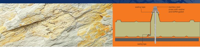
This sandwich panel with non-combustible insulation core rock wool meets today's high demands guidelines fire protection. According to the for non-combustible industrial construction, insulation materials are obligatory, particularly for large-surface and multi-storey buildings. For core thickness of 100 mm and higher a fire resistance up to 90 minutes can be reached. Additionally Hipertec® Roof panels show exceptional acoustic insulation behaviour as well. Thanks to the high quality of the
